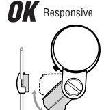
The round 'bump' on the sensor should not face the magnet.
